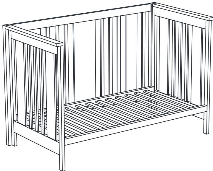
**Important:** If converting crib to Toddler daybed,make sure that the mattress support is in the **LOWEST** position.
