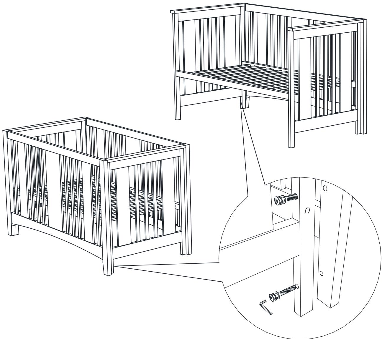
**Step 3:** In order to adjust the height of the mattress support, remove the 4 Allenhead Bolts(G) from the crib ends to the mattress support. Revise the height to the desired position,then reinstall the 4 Bolts. Tighten securely.
